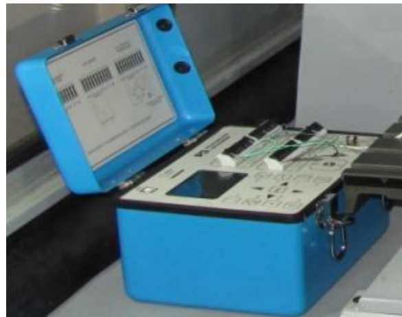
Fig.10. Data logger device for calling residual strains
