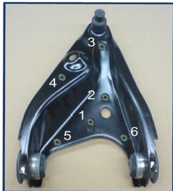
Fig.6. Position of rosettes installation
